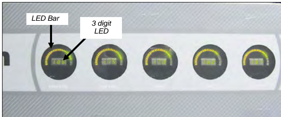
Close-up view of the display meters. Note the semi-circular indicator bars and the numeric readouts in the center.
