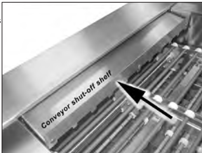
Shut-off shelf in the RUN position
