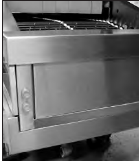
Load-end Start-Stop Station
