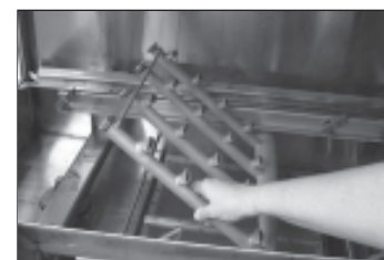
Figure 6- Lower Wash Arm Removal
