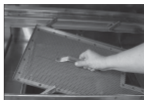
Figure 2- Scrap Screen Removal
