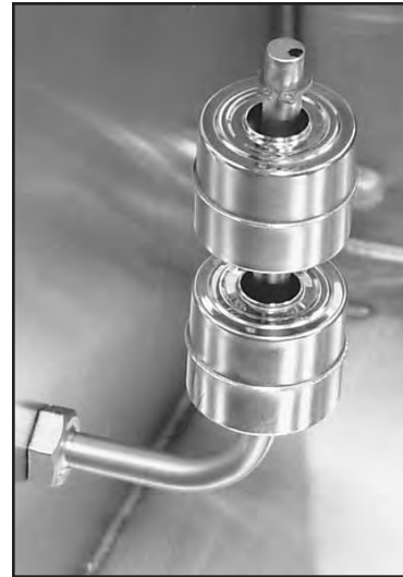
Figure 16 Dual Float Switch Assembly
