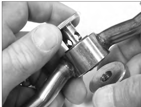
Disassemble the rinse arm assembly.
