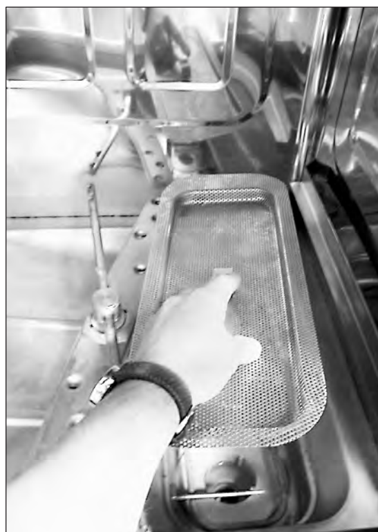
Make sure the scrap screen is in place.
