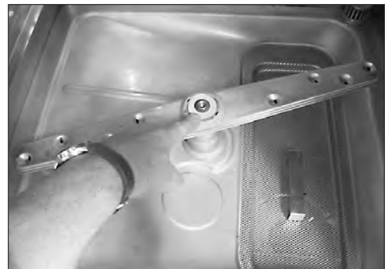
Clean the upper and lower wash arm bearings.
