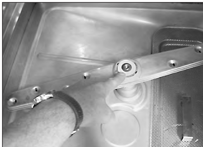
Clean the upper and lower wash spray arm bearings.
