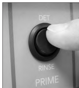
Push UP and HOLD until the detergent enters the wash tank compartment then release the push button.
