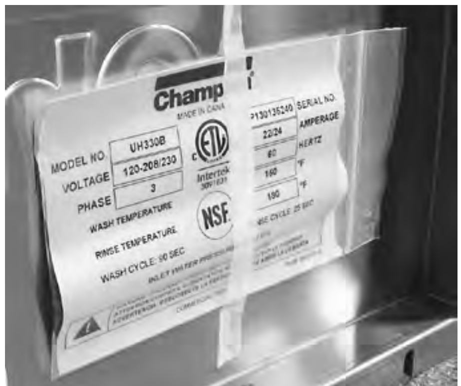
A three phase data plate is located on the back of the lower front panel.
