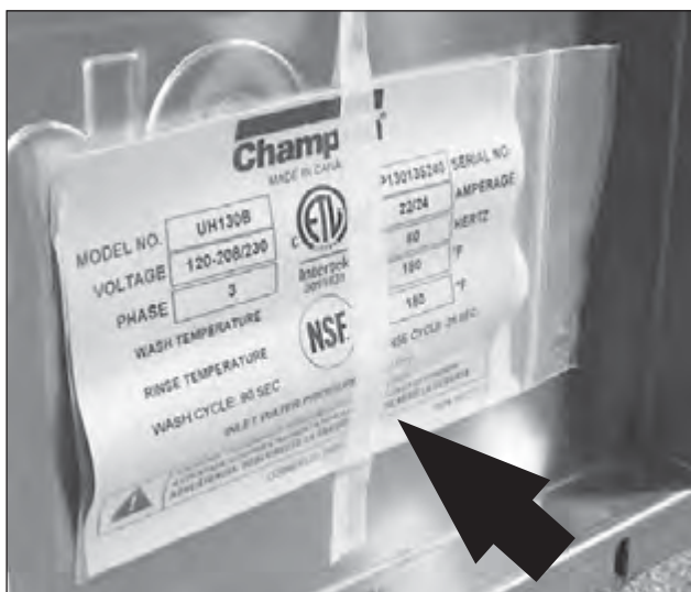
A replacement three phase data plate is stowed on the back of the machine lower front access panel.
