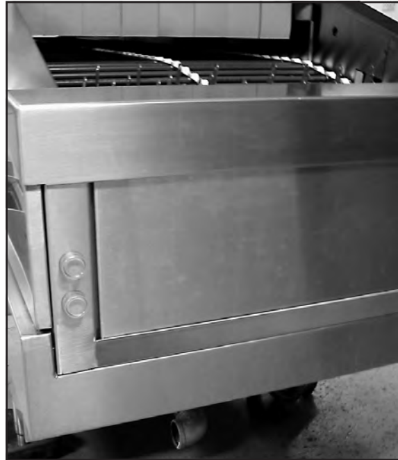
Load-end Start-Stop Station
