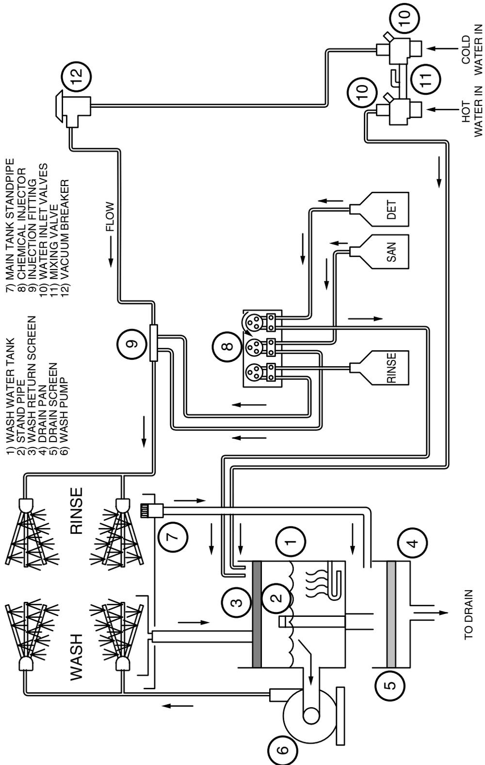
Figure 4 — Plumbing Diagram
