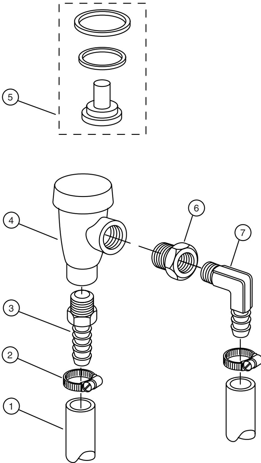
Figure 16 — Vacuum Breaker Plumbing
