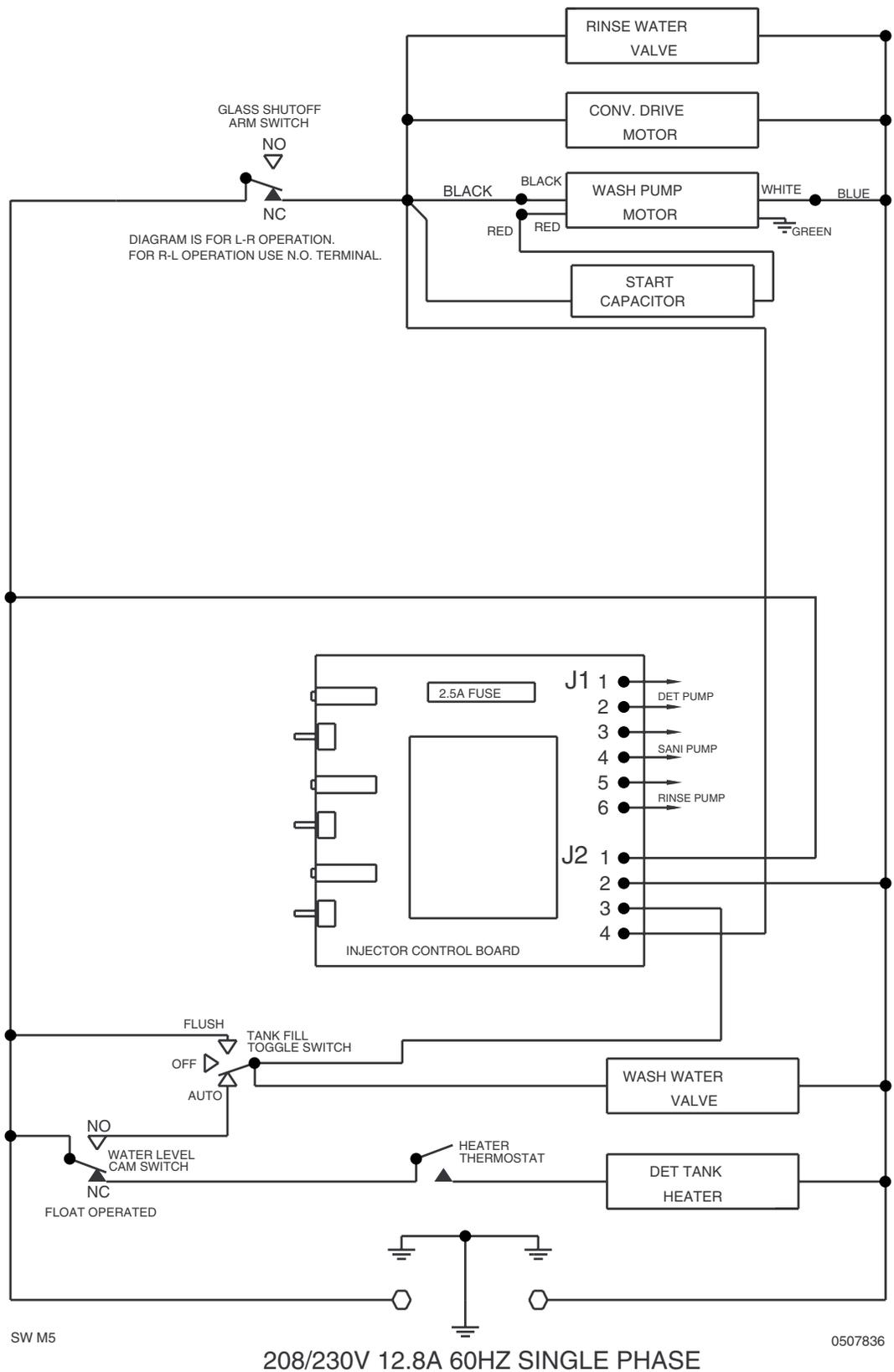
Figure 20 – Electrical Diagram (S/N 5181 through 6105)
