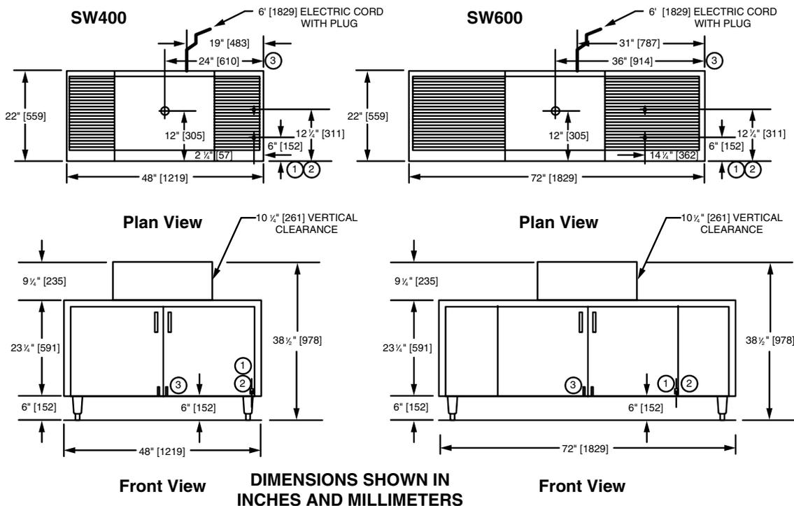
Figure 2 — Machine Measurements
