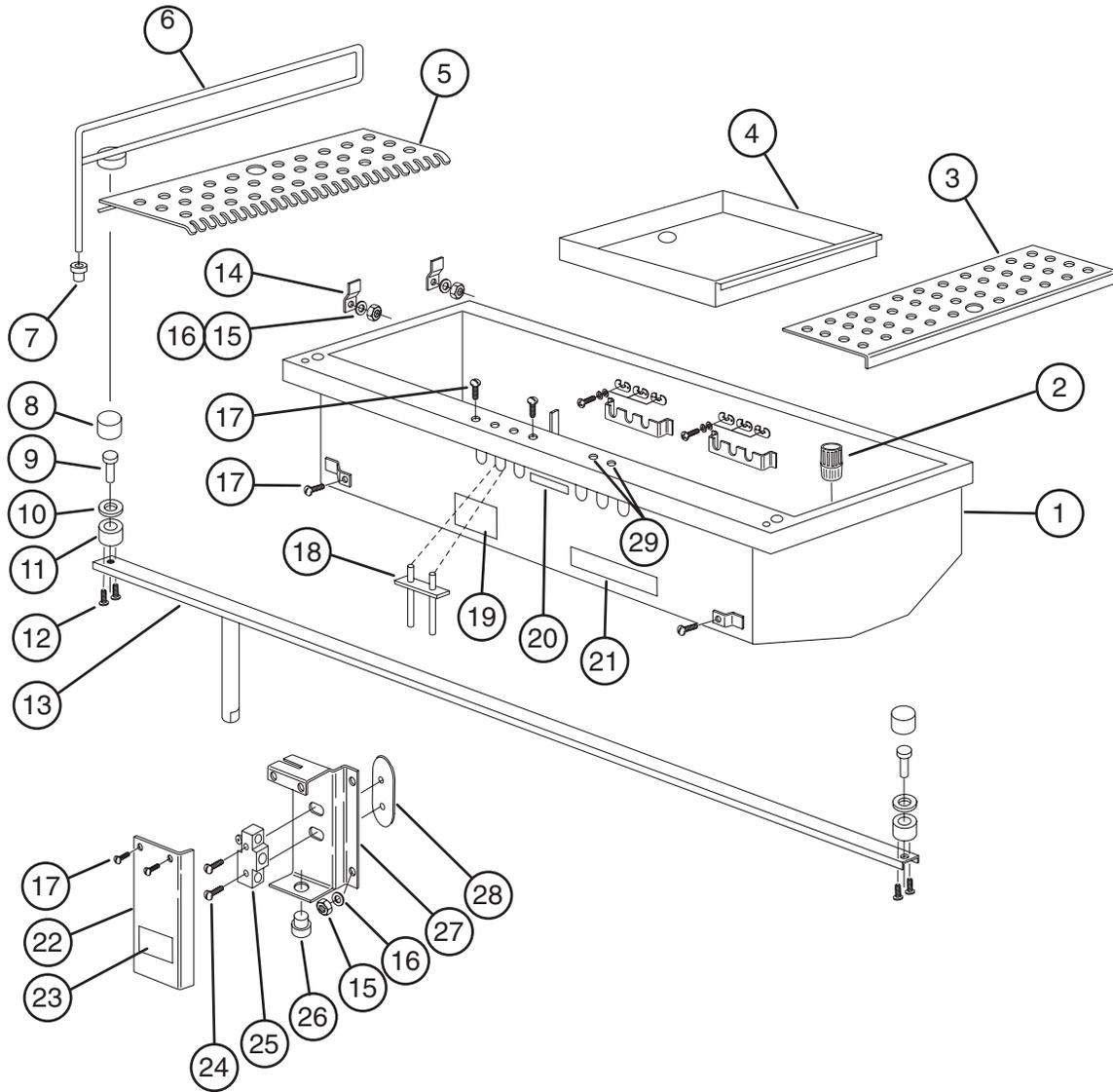
Figure 7 — Main Tank Assembly (R-L Shown)
