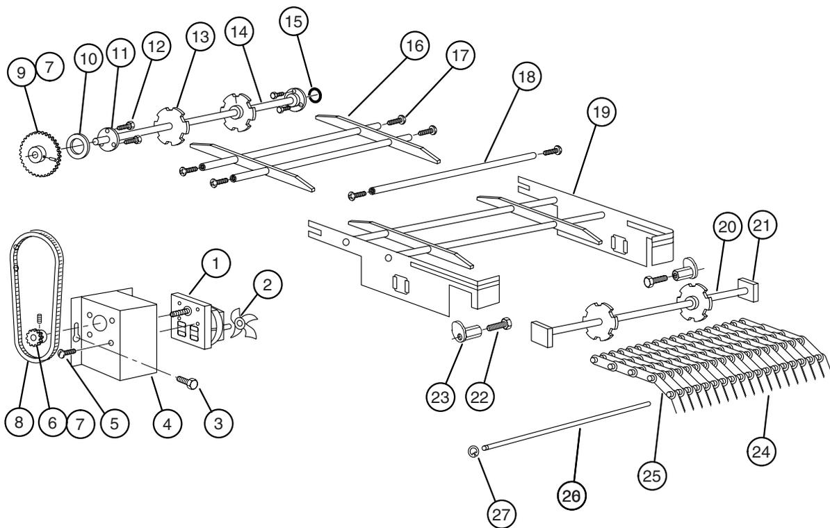
Figure 8 — Lift Bracket and Drive Assembly
