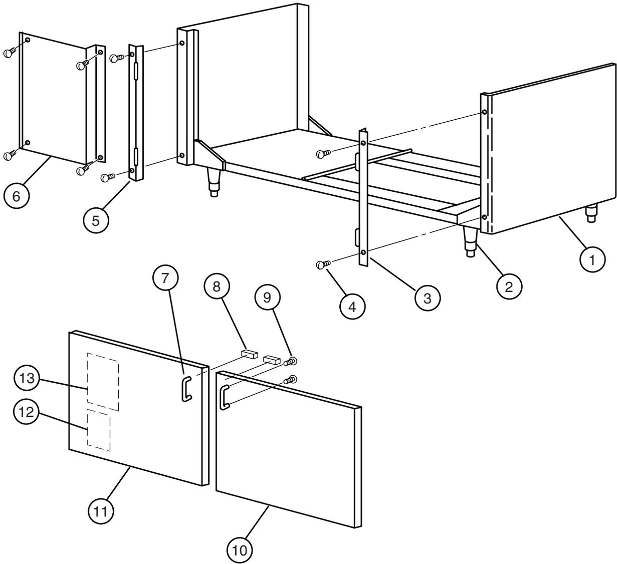
Figure 5 — Main Frame Assembly
