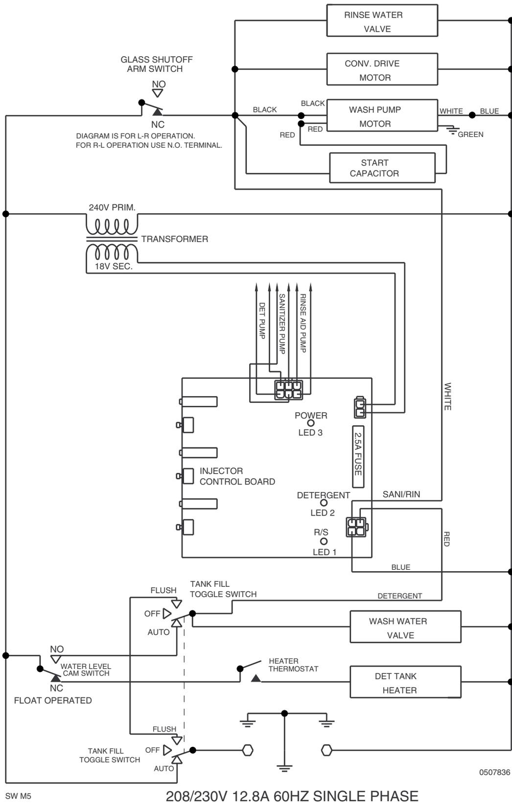
Figure 22 – Electrical Diagram (beginning with S/N 6216)
