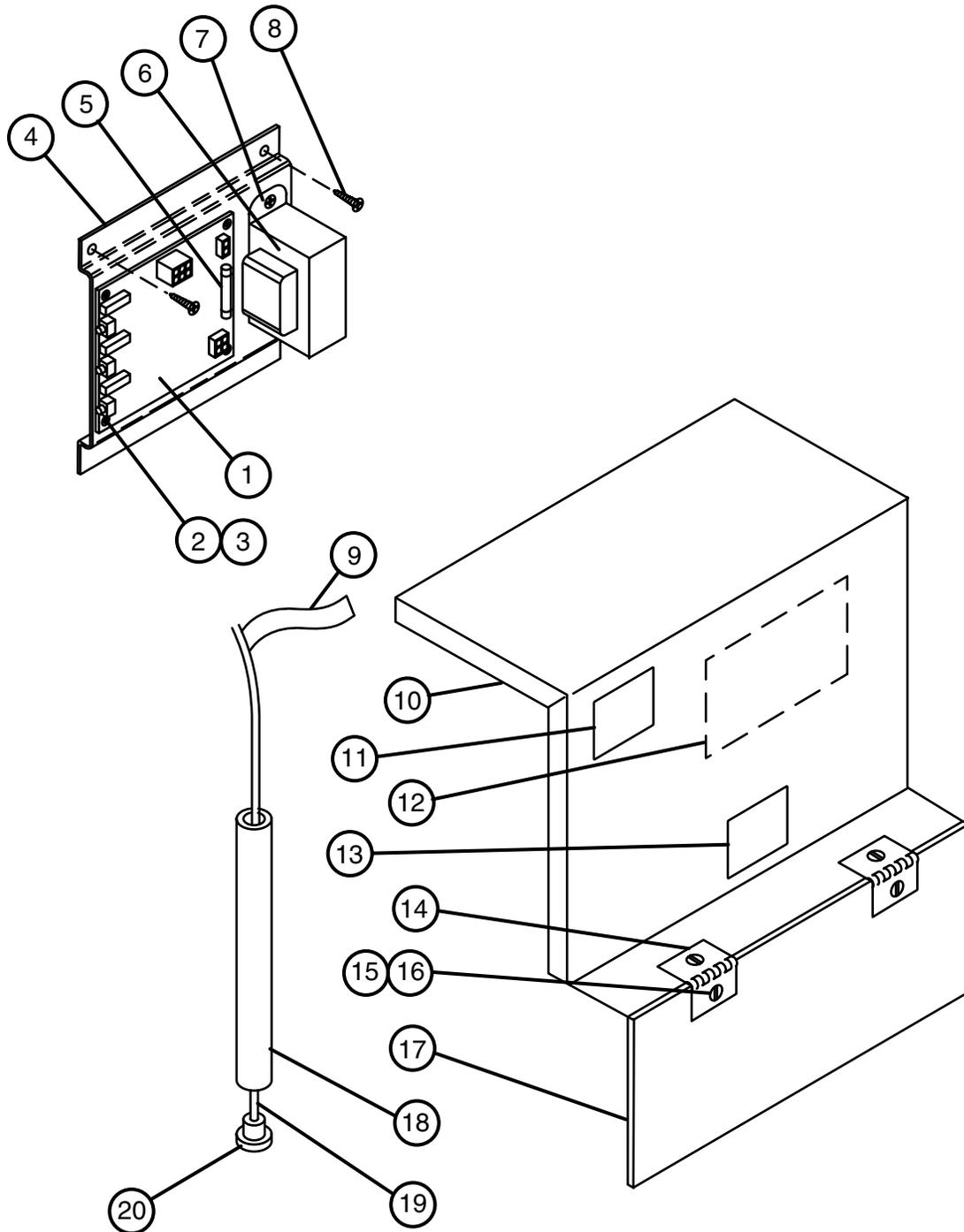
Figure 12 — Control Box Cover/Chemical Injector Board
