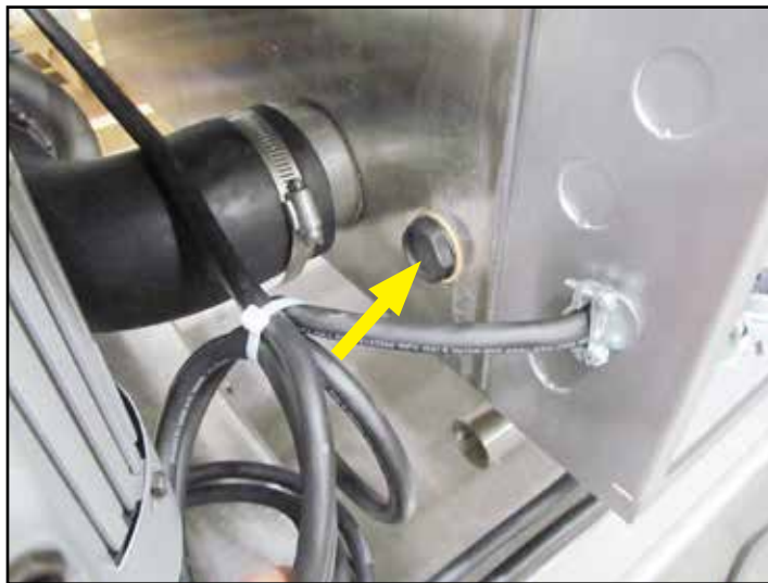
Fig. 19 - Detergent Sensor provided in side of wash tank.
