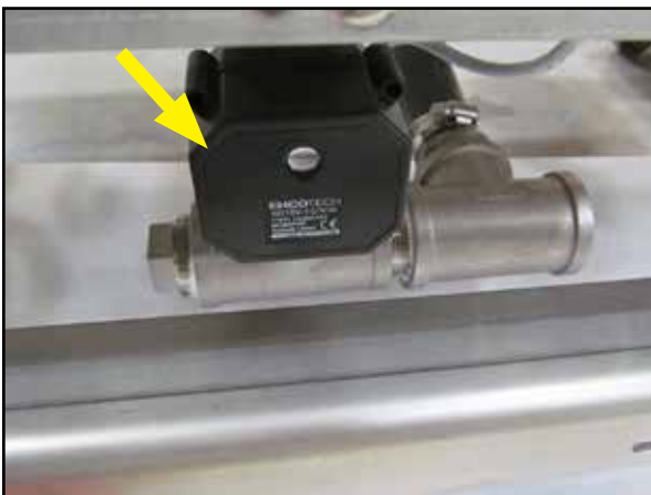
Fig.12 - Electric Drain Valve.
