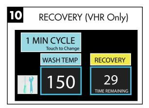
'RECOVERY' appears as heat and steam are removed from the wash chamber.
