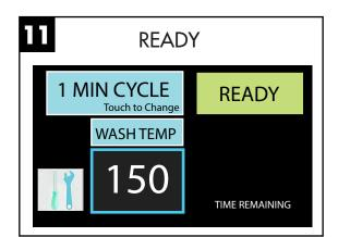
'READY' appears at the end of the cycle. Open the door and remove the clean wares.
