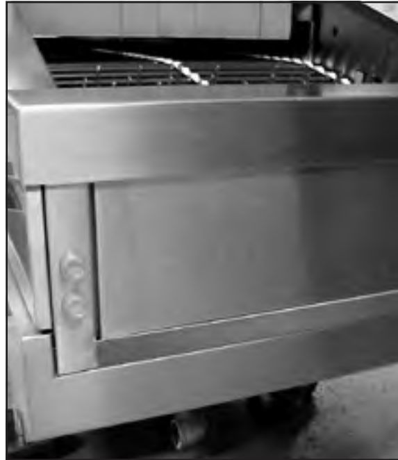
Load-end Start-Stop Station
