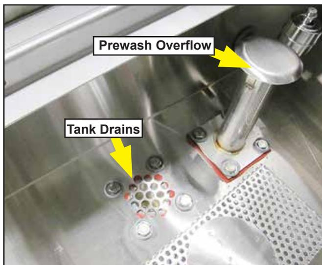
Fig. 72 - Tank drain prewash overflow
