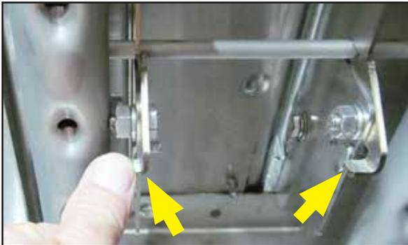
Fig. 64 - Press latches to release upper spray arm.
