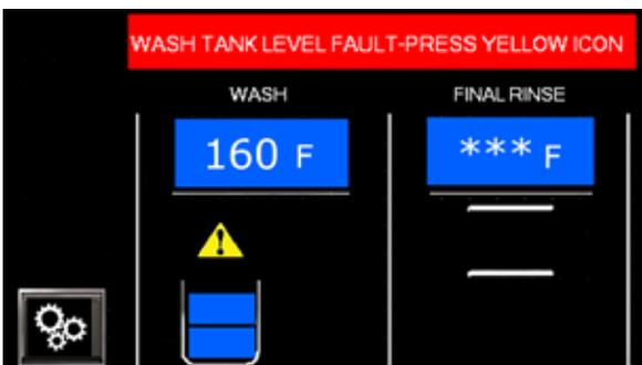
Fig. 25 -Wash Tank Level Fault
