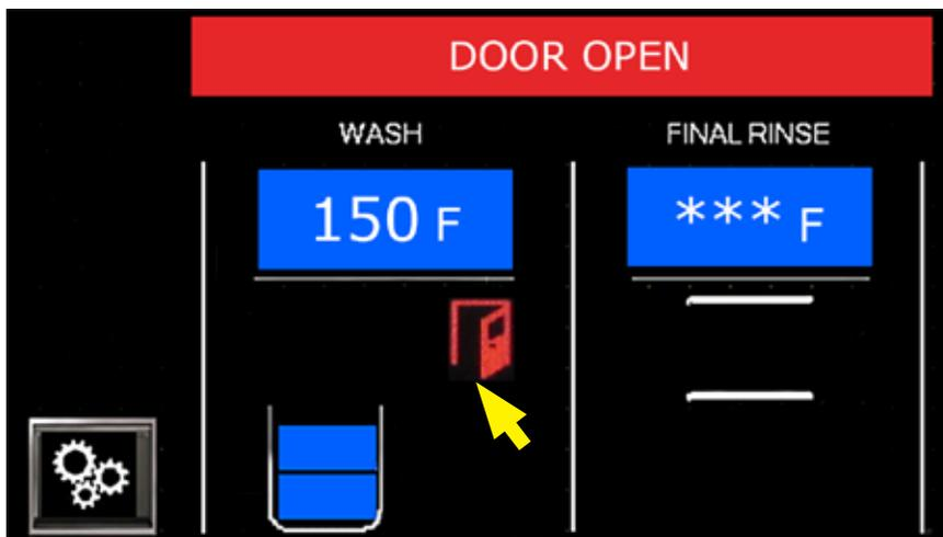
Fig. 22 - Door Open Fault
