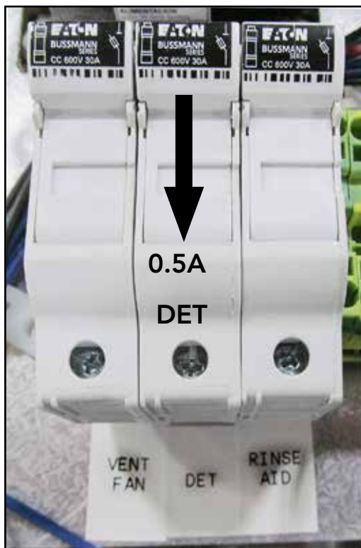
Fig. 18 - Connection is located inside the top control cabinet.
