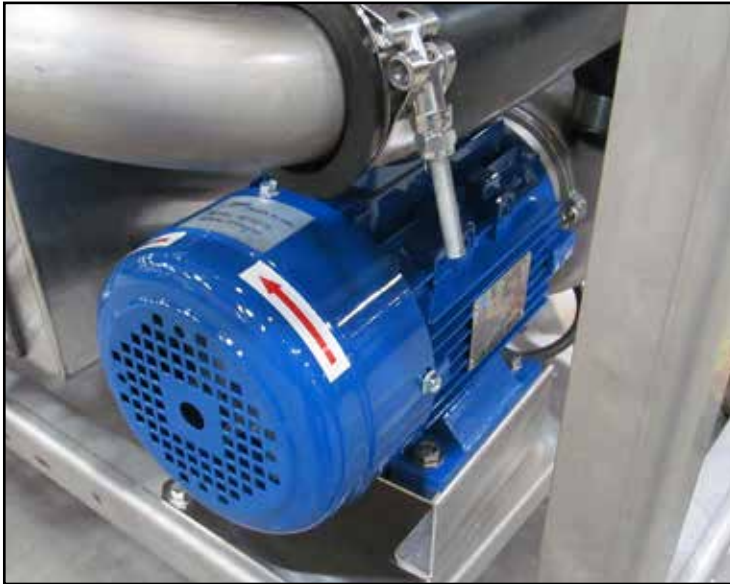
Fig. 26 - Motors rotate counter-clockwise.
