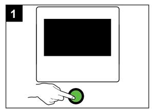
Push the power button OFF to automatically drain the machine.
