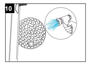
Flush the bottom of the tank making sure the drain screen is clear.
