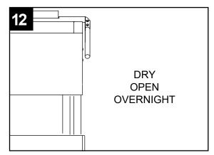
Reassemble machine and leave door open to aid in overnight drying.
