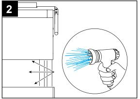
Spray the interior of the machine with fresh clean water.
