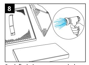
Back flush the screens and plate in a remote sink. DO NOT strike the screens against hard objects.
