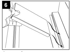
Remove the scrap screen support filler plate.
