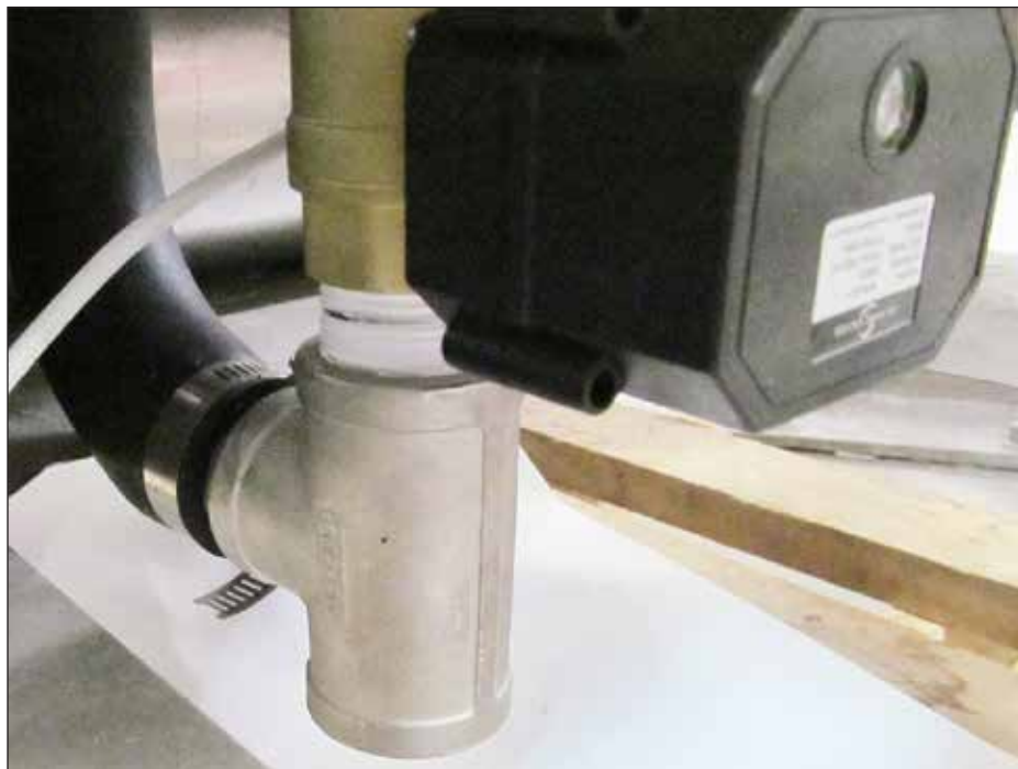
Fig. 7 - 1" NPT electric drain valve connection
