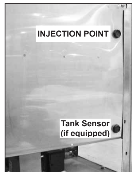
Fig. 18 - Injection and tank sensor (if equipped).
