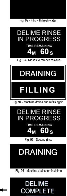
Fig. 97 -Fig. 97 -Delime operation is complete. Return to main screen.
