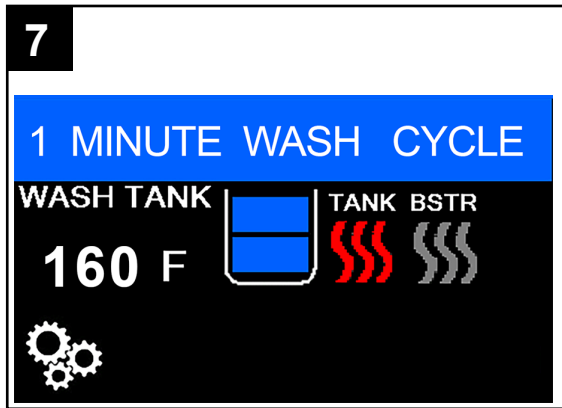
7 '1 Minute Wash Cycle' selected. Load wares Close door, red door icon disappears. Cycle begins.
