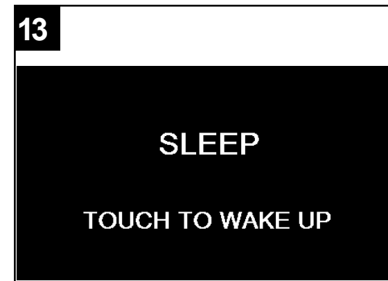
'SLEEP' appears if machine is idle for extended time. Touch the screen and the machine wakes up.
