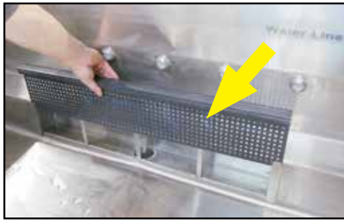
Fig. 12 - Install wash tank pump screen.
