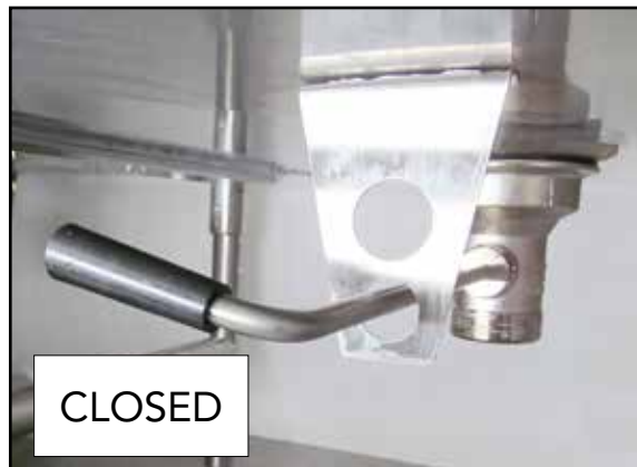
Fig. 6 - 1-1/2" NPT tank drain valve. Twist lever shown closed.
