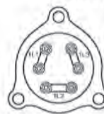
208-240V/3 Phase Delta Connection
