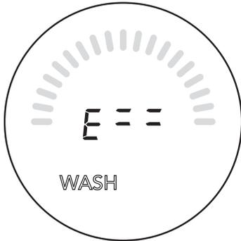
Indicates the wash thermistor is defective.
