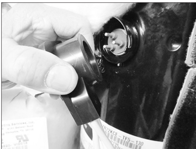
Fig. 7 - Connection is behind the insulation.
