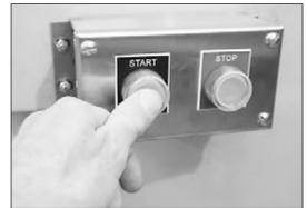
Push the START push button located on the water extractor.
