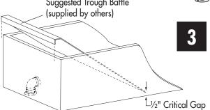
A splash baffle (supplied by others) must be fabricated and installed in the discharge end of the trough to create the proper water flow. See No. 3 at left for a suggested design for the baffle.
