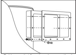
Rubber gasket for a trough connection is supplied with the pulper.
