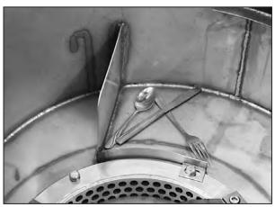
A powerful magnet is in the pulper grinding chamber. The magnet will attract utensils and other metal objects if they contain enough iron in their composition.
