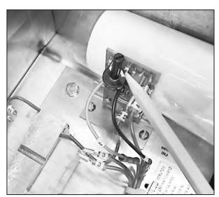
The Deodorizer Injector Speed Control Circuit board is located in the top left corner of the remote control cabinet.
