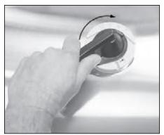
Turn the Main Circuit Breaker Switch to the ON position.
