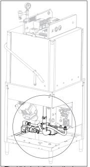
The kit is installed on the base of the machine.
