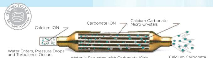
Water is Saturated with Carbonate IONs Carbonate Crystals are Grown on the Core Calcium Carbonate Crystals Exit the ION
