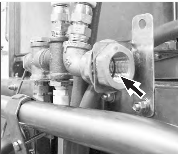
Fig. 8 - The COLD water supply is a 3/4" NPT connection located at the top left-side of the machine.
