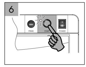
Close door, press and hold "START" button for 1 second and green in-cycle light will come on
