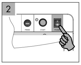
Flip "ON/OFF" switch to "ON" position
