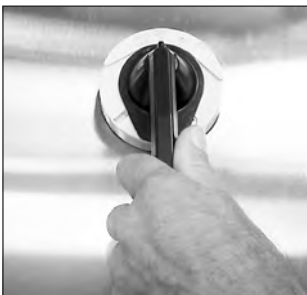
Main Circuit Breaker Switch in the OFF position
