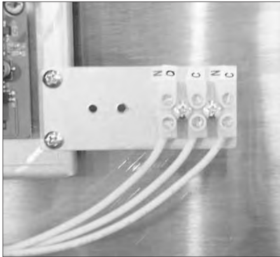
The Low temperature interlock block is located on the right-side of the booster cabinet interior.
