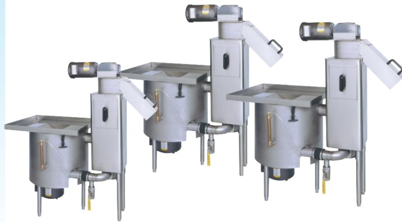
**P5-24** 24" pulper waste handling system. 5 HP grinder and 2 HP extractor motor handles 1,000 lbs/hour. Initial fill volume 18 gal. Slurry chamber and cutting disk. Configuration options.
