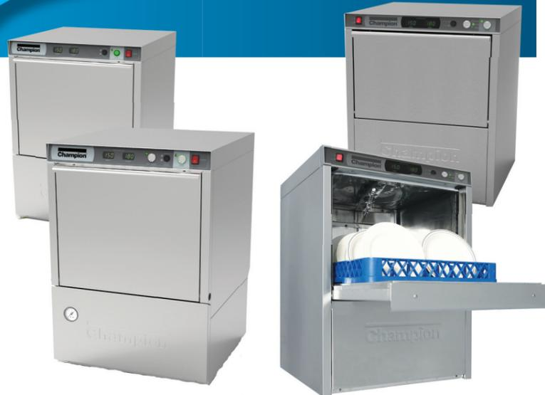
**UH130B** High temperature. Built-in booster heater. 25 racks/hour. 141 second cycle time. 1.8 gal/rack water consumption.
