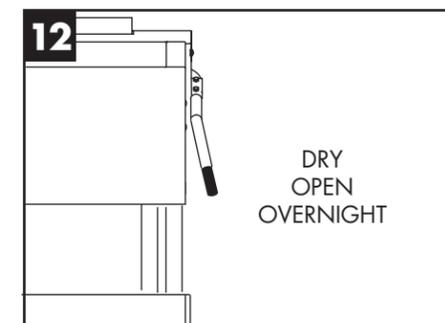
12 Reassemble machine and leave hood open to aid in overnight drying.
