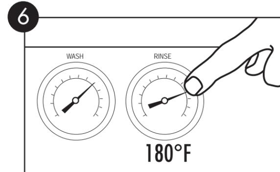
Check the final rinse temperature gauge during the final rinse. Minimum temperature 180°F/82°C.
