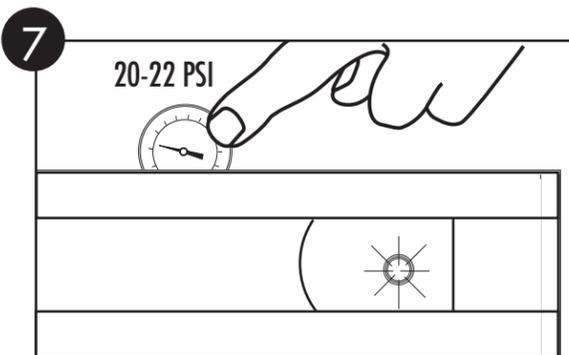
Check the final rinse pressure gauge during the final rinse. The gauge must indicate 20-22 PSI.
