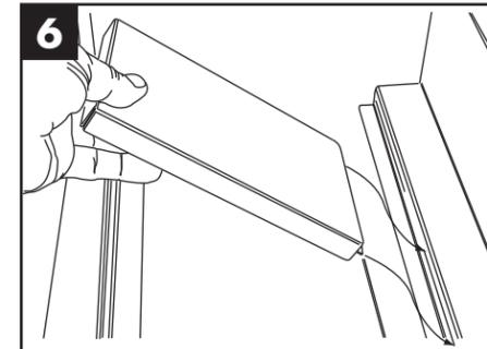
6 Remove the scrap screen support filler plate.
