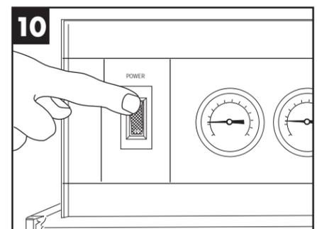
10 Push the power switch ON & immediately to the OFF position to drain.
