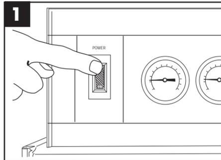
1 Flip ON/OFF switch to OFF position. The machine will drain automatically.
