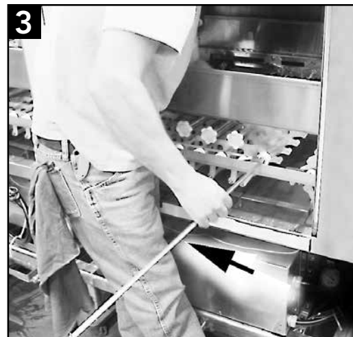
Connect the conveyor belt sections with a rod, spacers, and washers included in the hardware kit.
