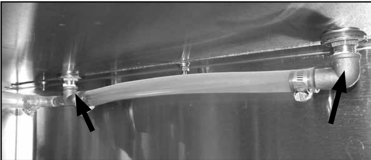
Fig. 20 - Connect flushing nozzle piping.
