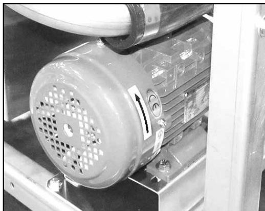
Fig. 25 - All motors are phased the same at the factory.
