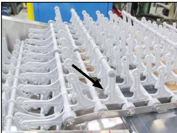
Fig. 5 - Belt peg notches face the load end.
