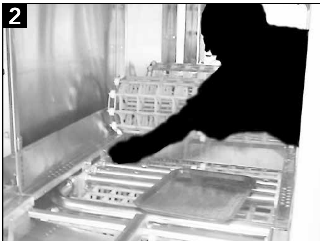
Roll the first section of conveyor belt from the unload section toward the load section.
